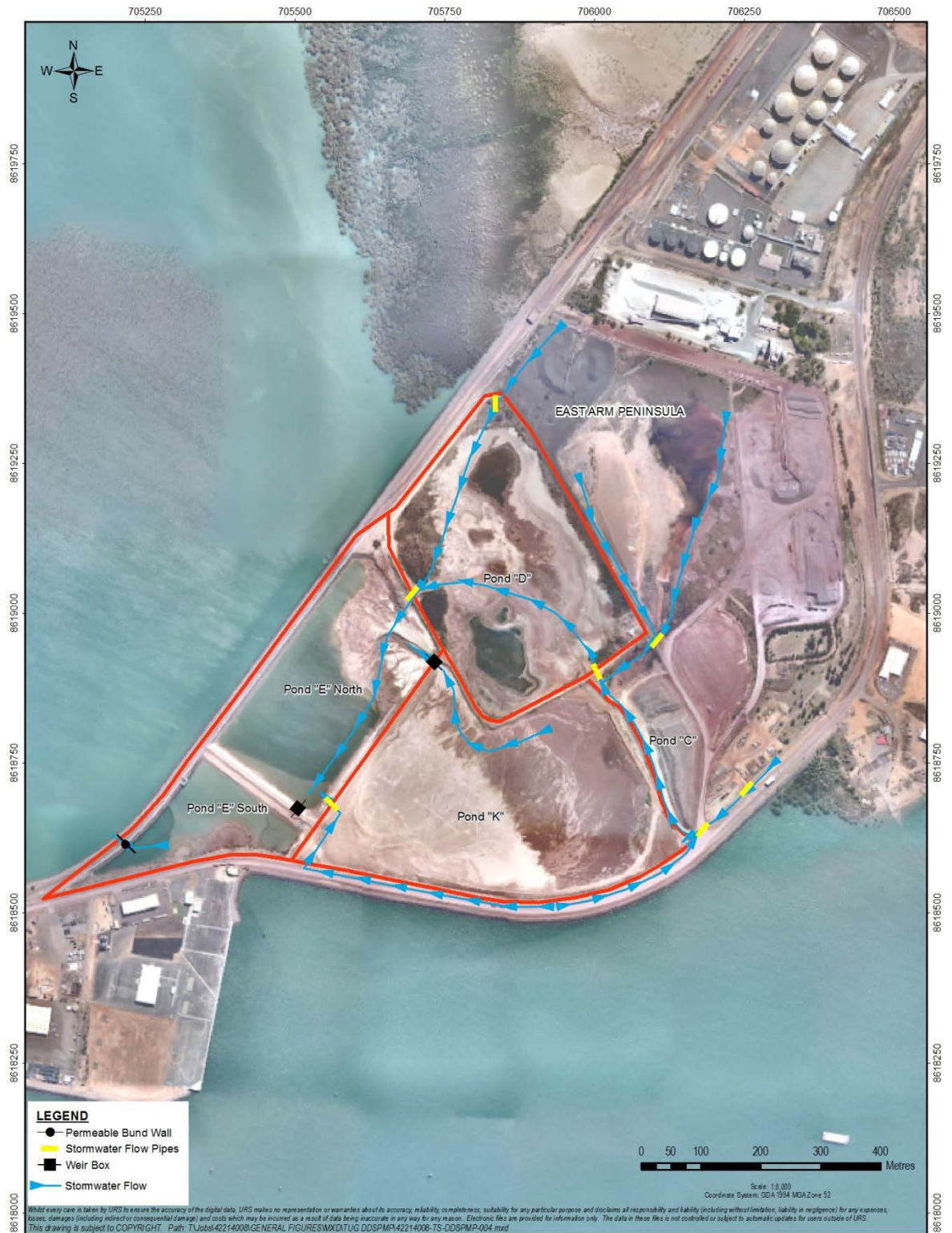
Figure 2-3 Water flow paths through EAW pond system
