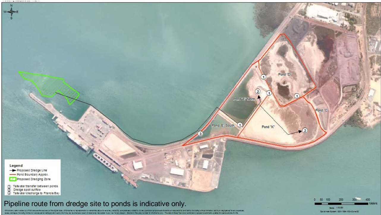
Figure 2-2 Placement of dredge spoil into EAW Ponds
