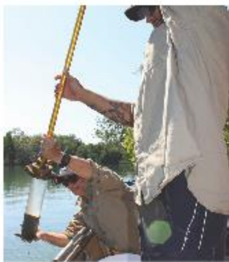
Julia Fortune and Matt Majid sampling in Short Creek - a tidal creek of the Elizabeth River. Cores are returned to the lab and placed within an incubation chamber with rotating magnetic stirrers to maintain ambient dissolved oxygen.
