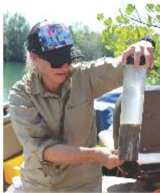
Julia Fortune and Matt Majid sampling in Short Creek - a tidal creek of the Elizabeth River. Cores are returned to the lab and placed within an incubation chamber with rotating magnetic stirrers to maintain ambient dissolved oxygen.
